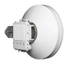
The SkyWay-EB-HP is Solectek's third-generation ULL PTP link operating in the 70/80GHz frequency band. It features the same 10ns latency per pass but now with a higher Tx output power of 25dBm at antenna port for more link budget and longer distances.
